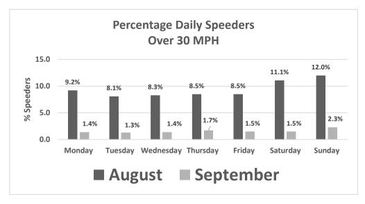
The installation of Speed Humps seems to have considerably reduced the percentage of speeders over 30 MPH.
