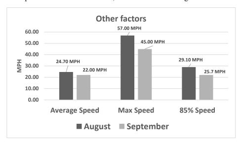
Average Speed Down, Maximum Speed Down, 85<sup>th</sup> Percentile Speed Down (85% of traffic is now at or below 25.7 MPH a big drop from 29.1 MPH in August) Full details of September traffic can be found on the website:
